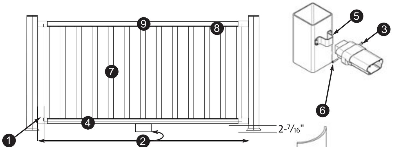
**NOTE:** Two brackets are required per section end.
