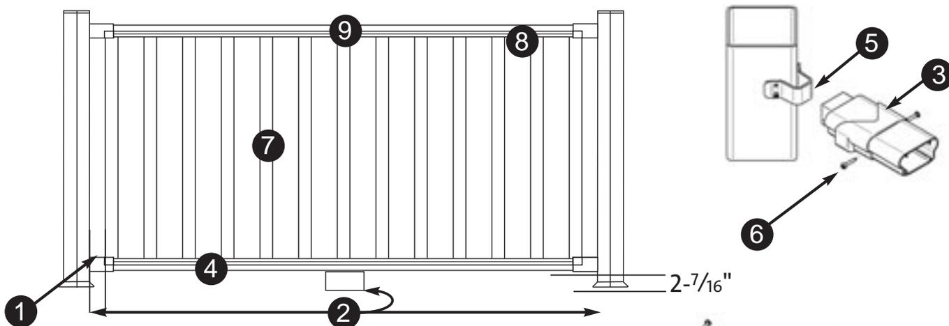
**NOTE:** Two brackets are required per section end.
